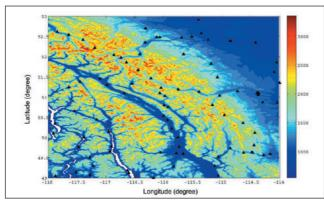
Figure 4: The topography map of the test area in Canadian Rokies. Elevations are supplied from SRTM3 database. Figures are given in meters. Triangles show GPS-levelling points.
