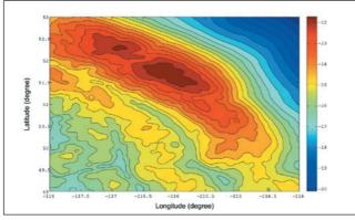
Figure 5: Combined Geoid over the test area. Values given in meters.
