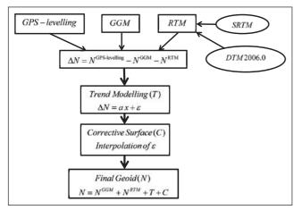
Figure 3: Computation scheme of geoid modelling procedure
